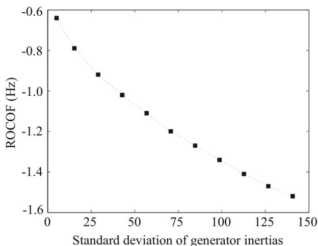
**Fig. 2** Change of the ROCOF with the dispersion of the distribution of the inertia contributions in the IEEE 39-bus system under the fault at bus 39
