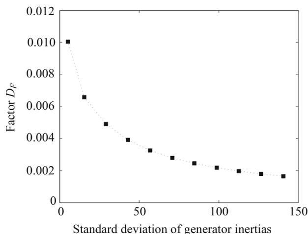
**Fig. 3** Change of factor  $D_F$  with the dispersion of the distribution of the inertia contributions in the IEEE 39-bus system under the fault at bus 39
