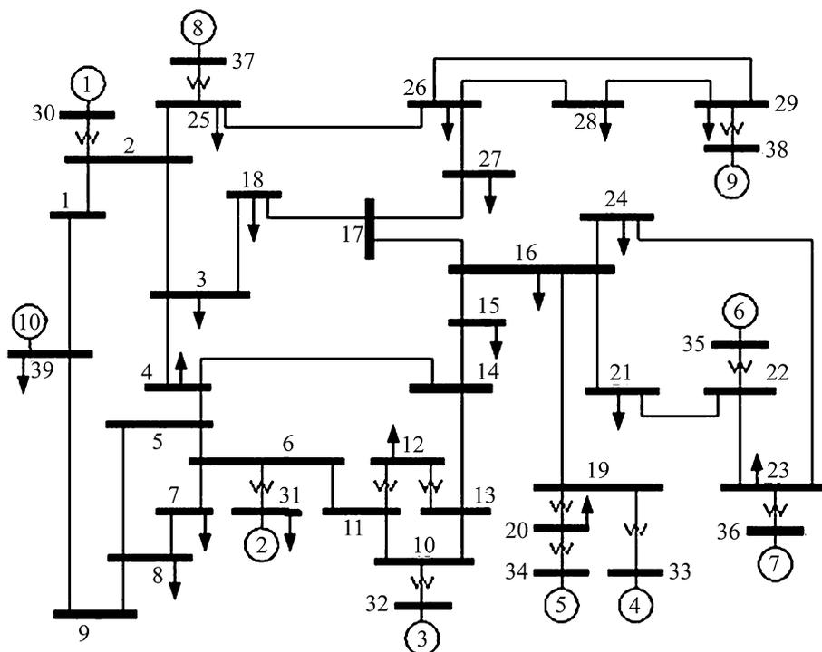
Fig. 1 One-line diagram of the IEEE 39-bus system
