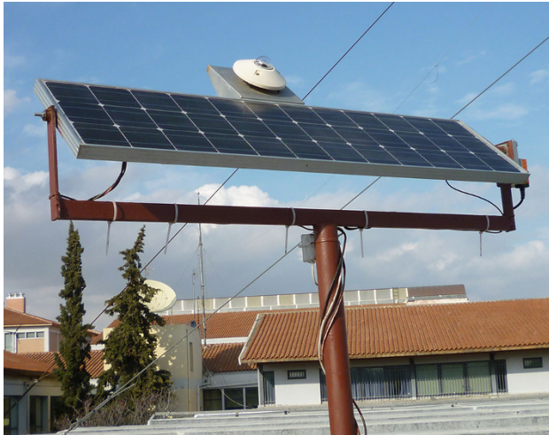
Fig. 1 PV panel, motorized mount and pyranometer configuration on the rooftop of the lab
