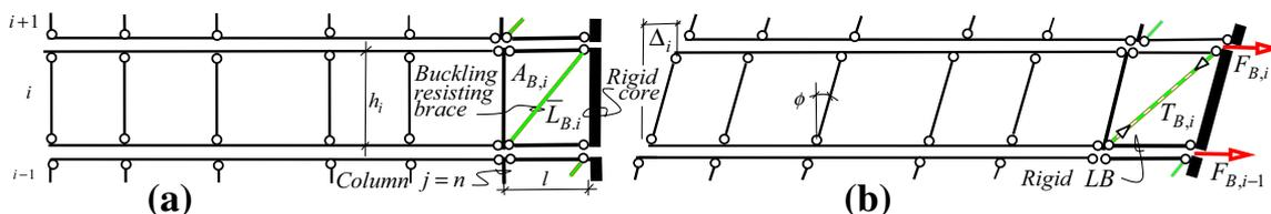
Fig. 5 a Subframe  $i$  and BRB before rotation, b subframe  $i$  and BRB after rotation
