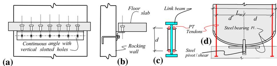
**Fig. 3** a, b Conceptual wall-slab shear connection, c link beam section, d rocking wall base and cables
