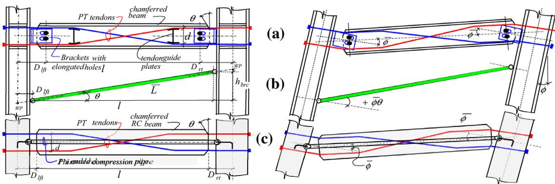
**Fig. 2** a Chamfered steel LB before and after rotation, b BRB before and after rotation, c chamfered reinforced concrete LB before and after rotation. (Reinforcing bars and other details not shown for clarity)
