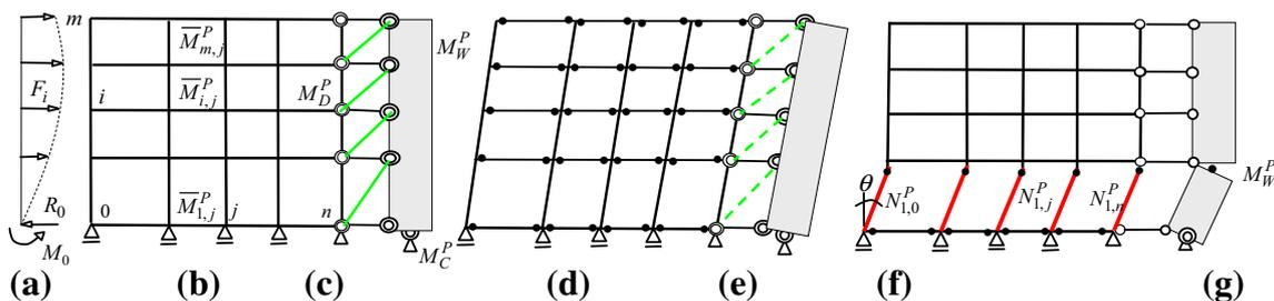
**Fig. 6** a Loading, b proposed dual system, c RRW, d MF failure, e BRB failure, f soft story failure of MF and g soft story failure of RRW. It should be noted that well-proportioned moment frames of RWMF are designed to fail in a purely sway mode as opposed to
