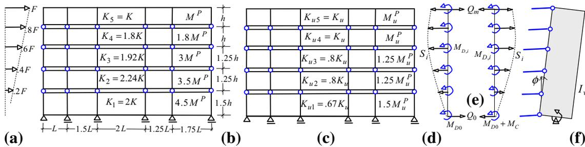
**Fig. 7** **a** Loading, **b** MFUR subframe stiffnesses and beam plastic moments, **c** MFUS subframe stiffnesses and beam plastic moments, **d** interactive forces acting against the MF and **e** Interactive forces acting against the RRW
