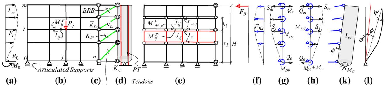
**Fig. 1** a A lateral loading, b grade beam restrained moment frame, c link beams, d rigid rocking wall, e equivalent subframes, f buckling restrained brace shear distribution and equivalent forces, g link beam
