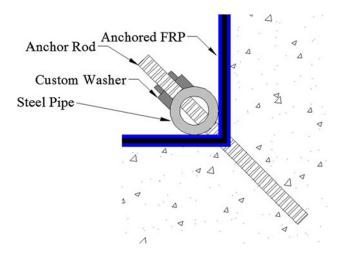
Fig. 11 CHS anchorage (adapted from Hiotakis 2004).
