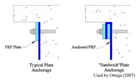
Fig. 9 Plated anchorage types.
