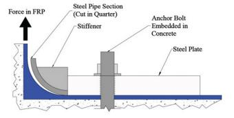
Fig. 13 Anchorage system studied in Grelle (2011).
