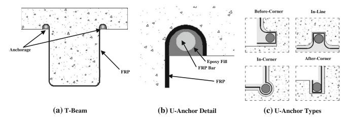
Fig. 6 Schematic of typical U-Anchor (Grelle and Sneed 2011).
