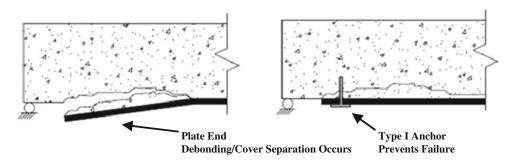
Fig. 2 Example of Type I anchorage device.
