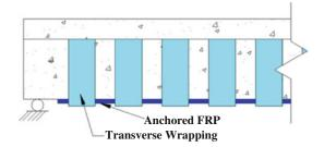
**Fig. 5** Example of transverse wrapping anchorage on T-beam.
