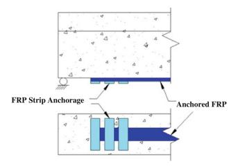
Fig. 8 FRP strip anchorage.
