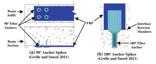
Fig. 4 Comparison of 90° and 180° anchor spikes.
