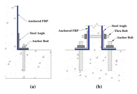
Fig. 10 Bolted angle systems.
