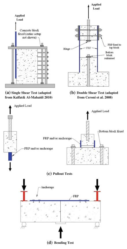
Fig. 15 FRP anchorage testing types.
