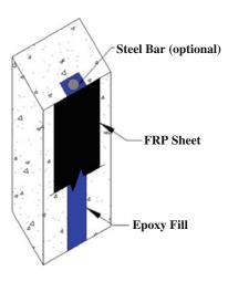
Fig. 7 Longitudinal chase anchorage used by Kalfat and Al-Mahaidi (2010).
