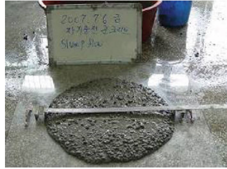
(b) Slump flow test for SCC
