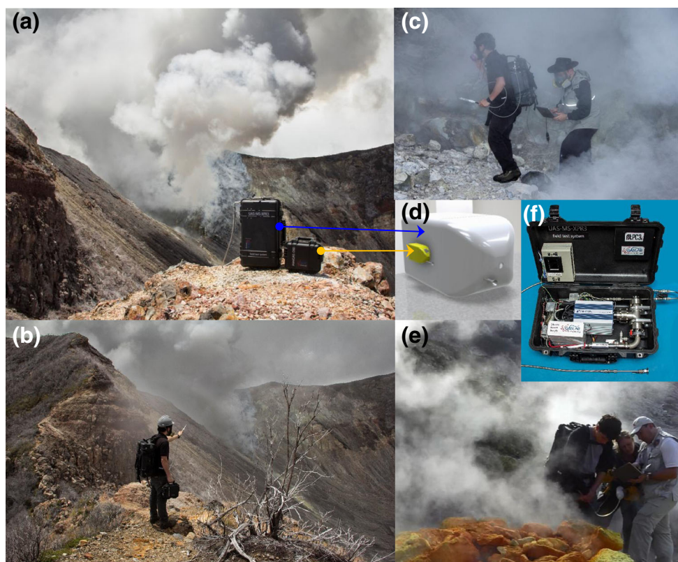
Figure 4. UAS-MS field test system deployments. (a) Turrialba volcano test site with both MiniGas and UAS-MS-MPH field test systems shown at the summit crater. The combined payloads are capable of acquiring geo-referenced trace gas concentration data for a large number of gases with a dynamic range, selectivity, accuracy, and repeatability that only a mass spectrometer can provide. It also measures independently \text{SO}_2 , \text{H}_2\text{S} , and \text{CO}_2 gas concentrations for cross-referencing, and acquires relative humidity, pressure, and temperature data. These capabilities are very useful for a large number of environments for both NASA and commercial applications. (b) Both systems are contained and transported in sealed Pelican cases, and can be easily backpack- and hand-carried to the volcano for field evaluation before they are integrated into the SIERRA UAV payload nose as depicted in (d). Three weeks after this picture was taken, Turrialba volcano erupted, and a massive collapse greatly enlarged the vent area shown, as active degassing continued. (c) UAS-MPH-XPR3 field test system being deployed into Las Hornillas fumarolic site at Miravalles volcano in Costa Rica and (e) Bocca Grande and Bocca Nuova fumaroles at Solfatara volcano test site in Naples, Italy for volcanic plume emission analysis. (f) Field test system consist of the MPD mini turbo molecular pump, scroll pump, and controller integrated to very small and compact vacuum chamber where the XPR3 mass spectrometer is also attached via 2.75" CF flange. A compact sample delivery system allows the direct sampling of the volcanic gases while maintaining good vacuum inside the vacuum chamber and provides a very fast response time using a small KNF 83.3 bypass pump. The system is powered with 24 V LIPO battery (white brick on the lower left of the picture)
