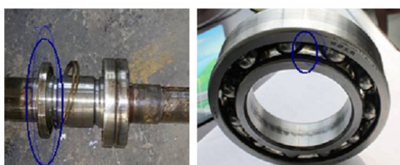
Fig. 15 Fault bearing physical picture.
