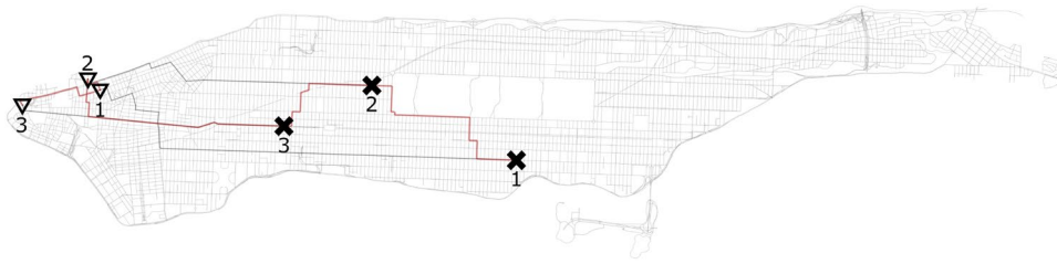
Fig. 1 Ride-pooling illustrated. Three travellers request to travel from their origins (marked with \times ) to destinations (marked with a \nabla ). Apart from offering them three separate solo rides (marked with grey), ride-hailing platform (like Uber) offers to pool them together
