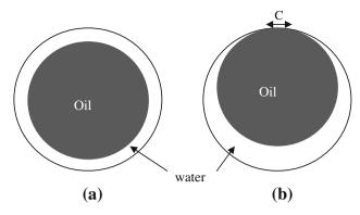
**Fig. 8** Radial position of the oil core: a perfect core-annular flow and **b** with density difference. *C* is the contact perimeter between the oil phase (core) and the pipe wall
