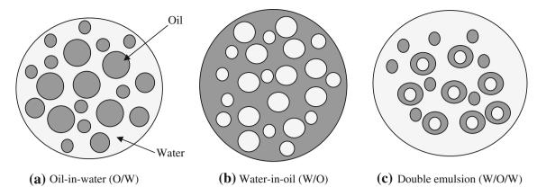
Fig. 5 The several emulsions that are used to transport heavy crude oil
