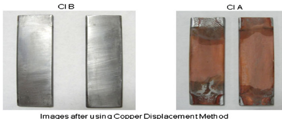
Fig. 5 Images of coupons treated with corrosion inhibitors CIA and CIB after the 24-h wheel test and the copper displacement test
