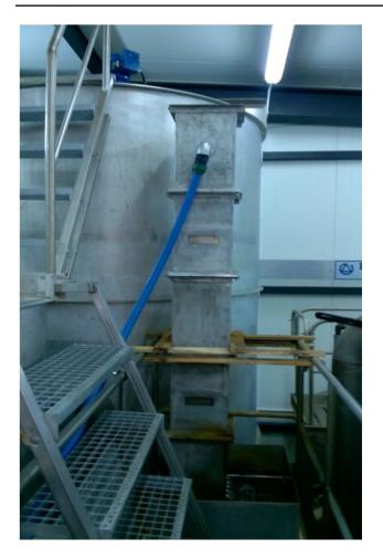
Fig. 2 Aerator for water aeration
