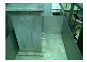
Fig. 3 Last segment of the aerator with aerated water outflow
