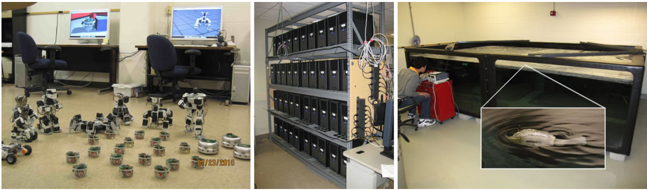
Fig. 1 Components of Evolution Park testbed: ( left ) collection of terrestrial microrobots and interactive simulation cluster; ( center ) rack-mounted parallel computing platform for evolution runs and behavior
