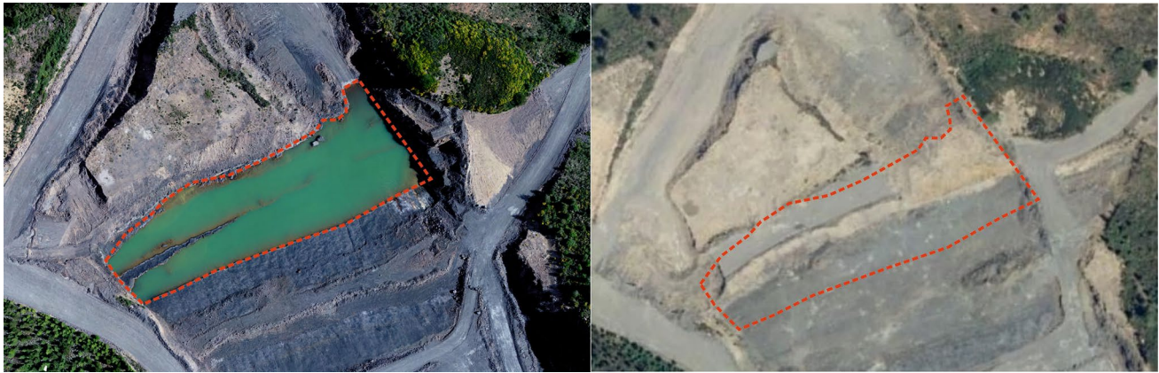
Fig. 2 Example of using a drone to make current orthophotograms. On the left, a recent (2020) drone-derived image of a mining pit lake in the Fabero area. On the right, the same pit lake in the available orthophoto (2017) from the Spanish National Geographic Institute (IGN)
