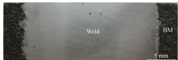
Fig. 11. Macroscopic image of the top surface of the joint after immersion in EXCO solution for 6 h.
