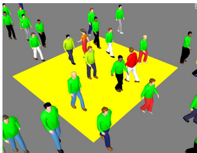
Fig. 2 Illustration of combined application of area-based and individual-based LOS value calculation. The pedestrians of the main walking direction experience a better LOS value (displayed as green and yellow-green shirts ) than is measured on the area
