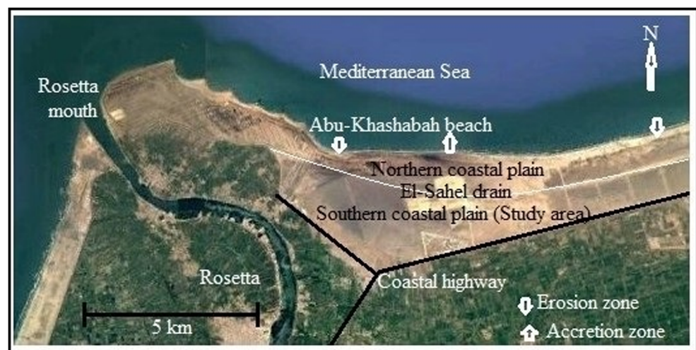
Fig. 2 Satellite photo showing the zones of erosion and accretion along the shoreline north of the study area
