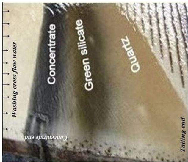
Fig. 8 Separation of economic heavy minerals using half-size Wilfley shaking table
