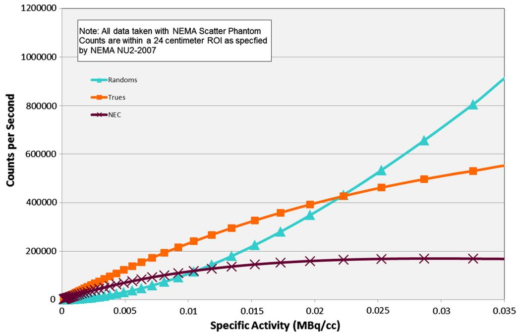
**Figure 2.** Count Rate Performance showing Biograph mCT TrueV reflecting the high count rate performance of the fourth ring. The increase in sensitivity may facilitate the use of lower doses of Rubidium-82 chloride in a combined MBF-MPI protocol.
