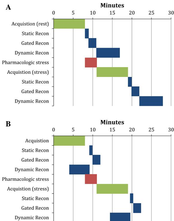
**Figure 4.** **A** Serial PET reconstruction that starts after the PET acquisition does not complete image reconstruction until 9 minutes post acquisition **B** Parallel PET reconstruction that starts in parallel with the PET acquisition completes the image reconstruction in less than 4 minutes post acquisition.
