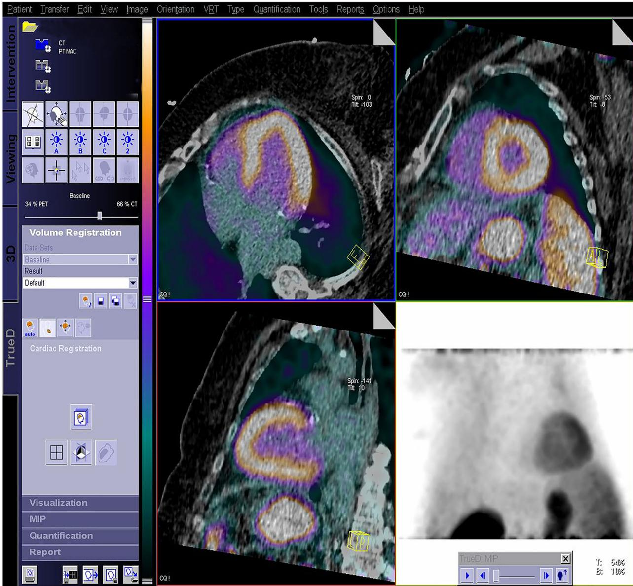
**Figure 3.** SMART Auto Cardiac Registration automatically aligns the non-attenuation-corrected (NAC) PET with the CT data in order to ensure optimal AC. The fused data is presented in transverse, coronal, and sagittal views. Data courtesy of University of Michigan, Ann Arbor, USA.
