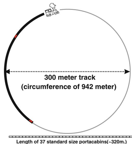
**Fig. 1** First approach for a large diameter human centrifuge. A 300 m. diameter centrifuge should be something like a train track system. The total circumference would be 942 of which some 320 m. would be occupied by e.g. 37 standard size portacabins (see also Table 1)
