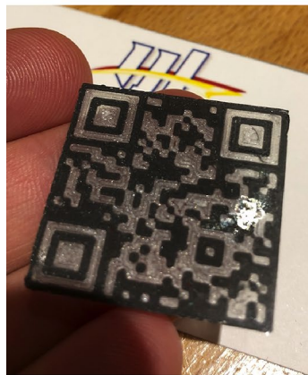
Fig. 10 Left: Anti-fraud label prepared by additive manufacturing of a polymer-matrix composite added with a blend of complex metallic alloy powders. The fingers show the approximate size of the device. It can be read directly with visible light, but its X-ray diffraction pattern is unique and therefore cannot be counterfeited. Right: Example of a piece of art entitled “In memory of us, la beauté du geste” by Stéphane Simon that will be on exhibition in Paris during the Olympic Games in 2024 and is labelled using a QR code as shown on the left (Courtesy of Samuel Kenzari, Institut Jean Lamour, Nancy, France)
