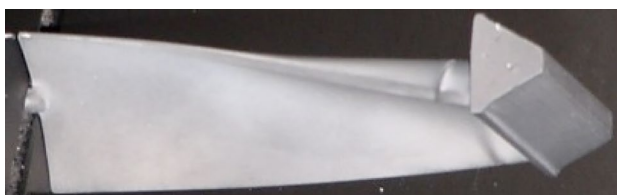
Fig. 14 Helicopter turbine blade equipped with a thermal barrier made of a hexagonal approximant of the decagonal quasicrystal that was deposited on top of the metallic substrate by PVD magnetron sputtering (Courtesy of S. Drawing, ONERA)
