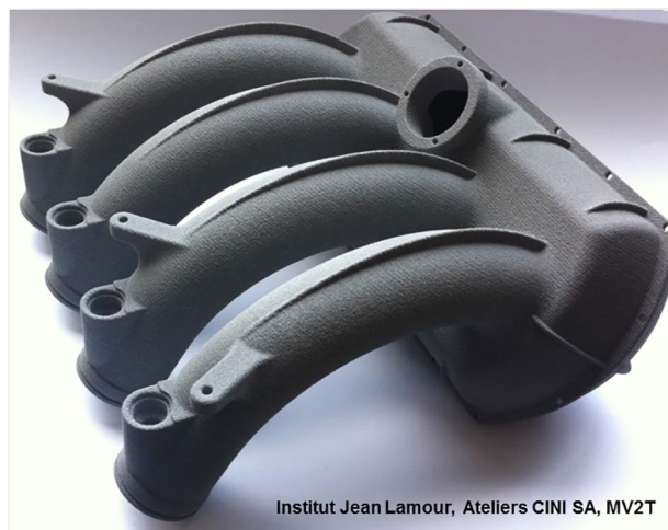
Fig. 7 Ensemble of exhaust pipes made by additive manufacturing of a polyamide powder loaded with atomised quasicrystalline grains (see Graphical Abstract) for a race car. The part is fabricated in one single step, in spite of its high complexity. No further surface treatment is required to make it tight to the exhaust gases (taken from Kenzari et al. 2012)
