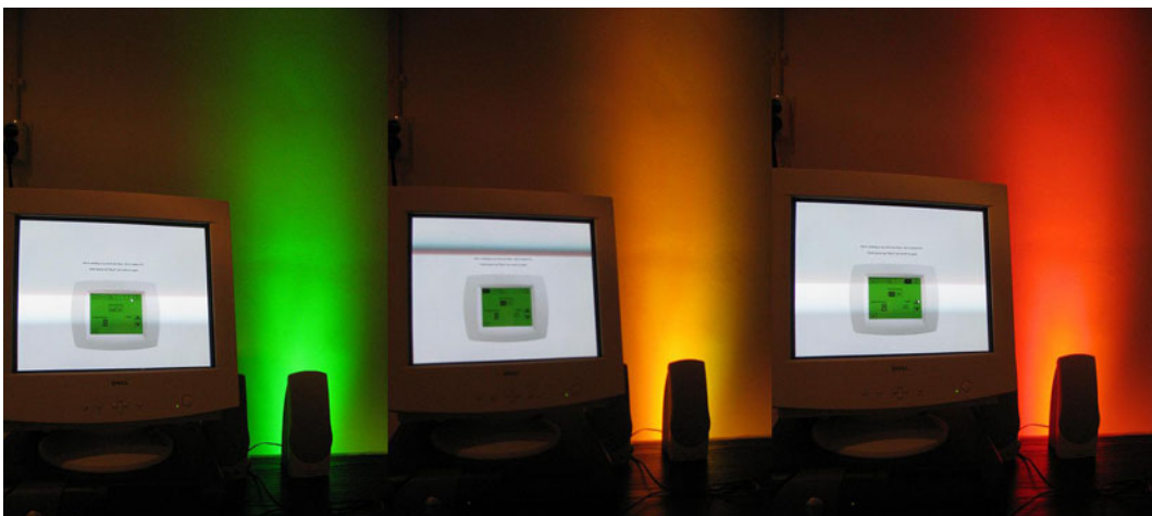
Fig. 2 A high power programmable LED lamp projecting light on the wall behind the participant’s desk indicating low (left picture), medium (middle picture), or high (right picture) energy consumption
