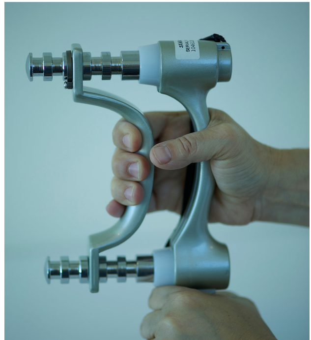
Fig. 1 Standard hand positioning for the instrumented digital dynamometer followed the American Society of Hand Therapists guidelines [21].
