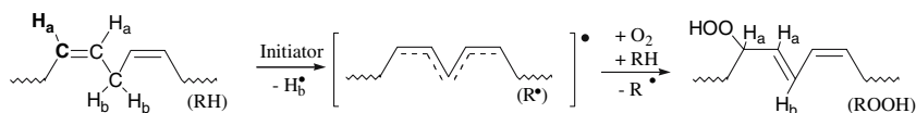
Fig. 3: The cis H_a-C=CH hydrogen of a 1,4-pentadiene unit in a fatty acid disappears in the first step of the autoxidation due to abstraction of a H_b atom and rearrangement of the resulting pentadienyl radical
