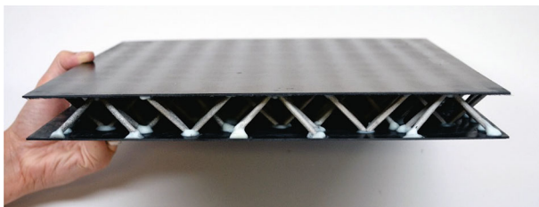
Fig. 9. Sandwich panels ( 30 \times 30 \times 3 \text{ cm}^3 ) with nanocrystalline Al-Mn truss core and CFRP facesheets fabricated for testing.
