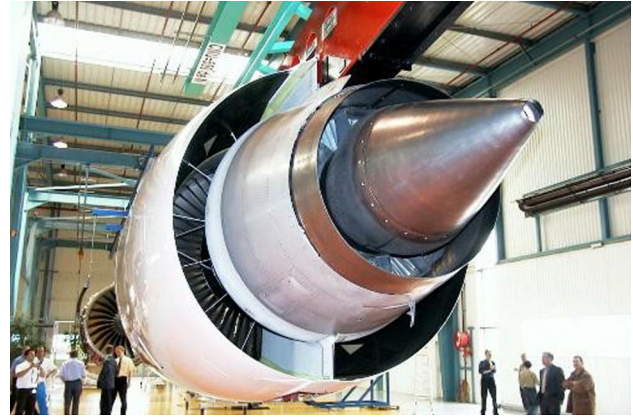
Fig. 18. Beta 21S plug-and-nozzle assemblies for the trent 500 engine on the Airbus A340-500/600 49 .
