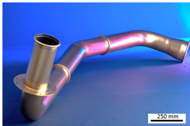
Fig. 11. Ti-15V-3Al-3Sn-3Cr welded environmental control system duct (photo courtesy of Exotic Metals, Kent, WA).
