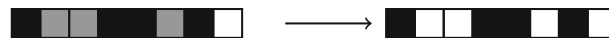
Fig. 4 An example of propagation implied by the second constraint in a row of length 8. Since the number of zeros is equal to 4, we can deduce that the remaining cells should be equal to 1
