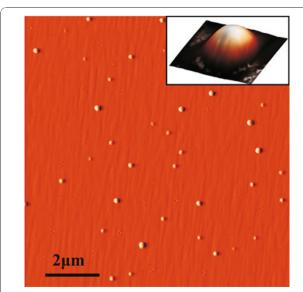
Figure 1 10  $\times$  10  $\mu m$  AFM image of GaAs substrate with indium droplets. The single droplet image 300  $\times$  300 nm is presented in the *inset*.
