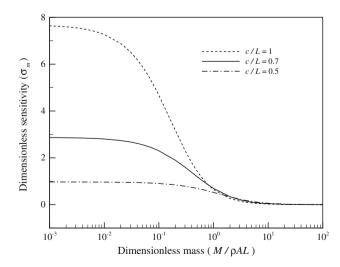
Fig. 5 The effect of location of attached mass on the sensitivity of the sensor for  $e_0 a/L = 0.3$
