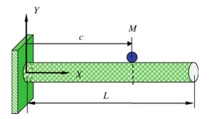
Fig. 1 A cantilevered nanotube-based mass sensor with an attached mass
