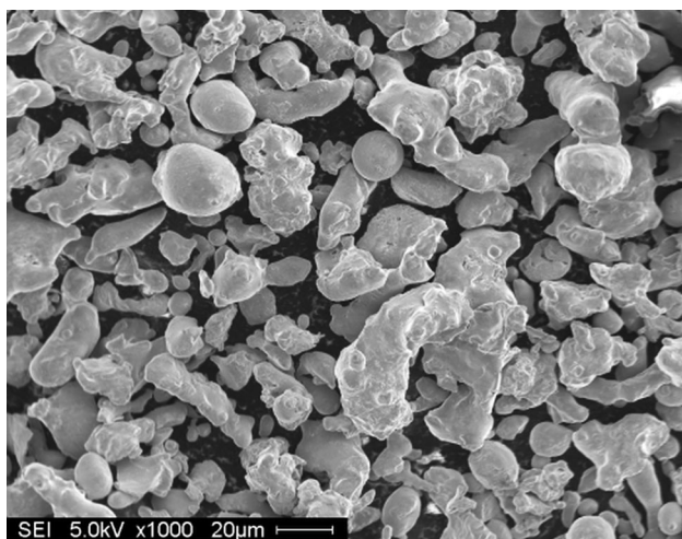
Fig. 2 SEM micrograph of 316L powder
