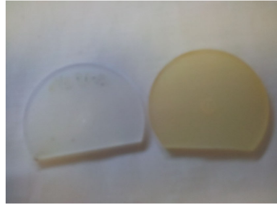
Fig. 11. Discoloration of BPA-PC after photo-thermal ageing at 140°C.
