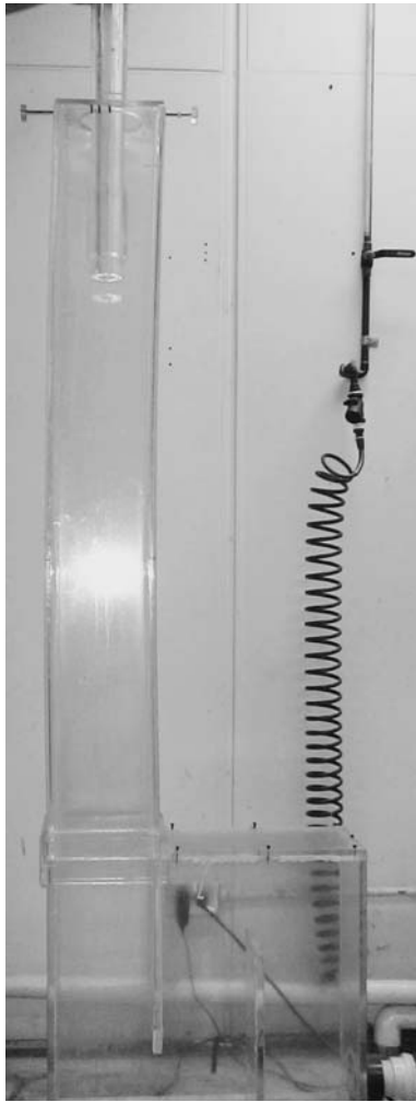
Fig. 7—Plastic mold model with the nozzle in the top.
