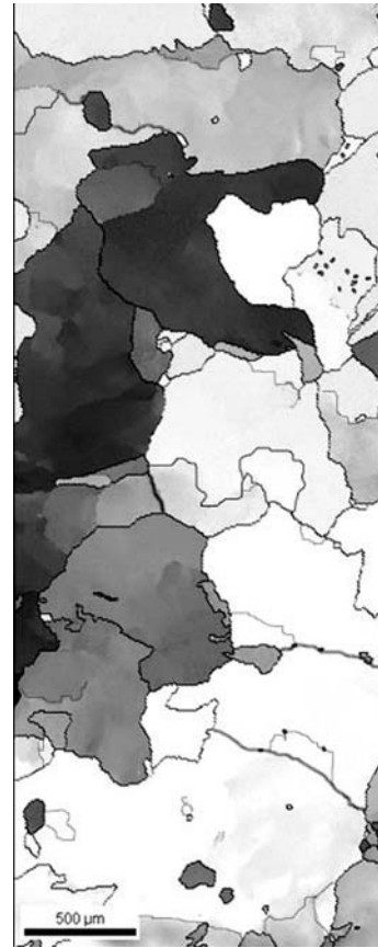
Fig. 5—High-angle grain boundaries (thick, black lines) and small-angle grain boundaries between subgrains (thin, gray lines) in the investigated Fe-0.005 at. pct N alloy after completed transformation (cooling rate of 10 \text{ Kmin}^{-1} ).
