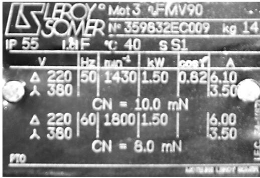
Fig. 12 Motor nameplate
