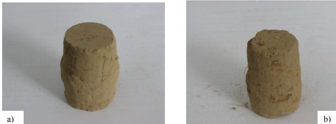
Figure 10 Triaxial tests of deformability for soil without roots and root-soil composite system samples; a) Soil without roots sample shape; b) A. canescens sample shape
