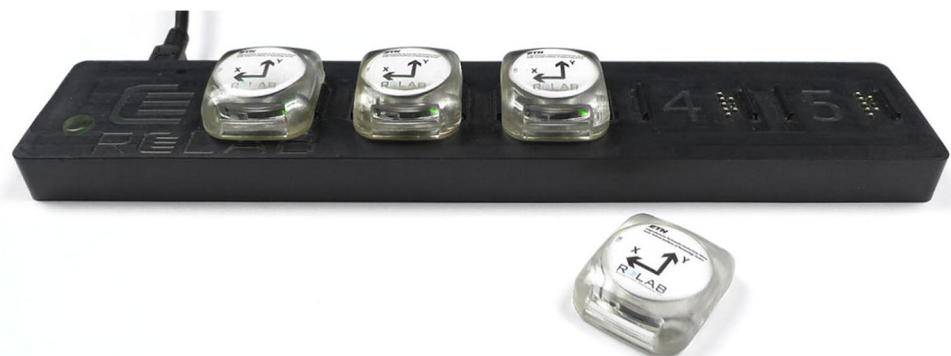
Fig. 1 ReSense sensor modules and base station [14]. The base station allows data readout, battery charging and temporal synchronization of up to 5 sensor modules simultaneously via a USB 2 port
