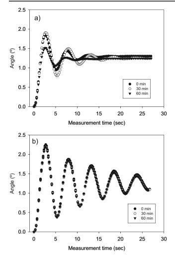
Fig. 3 Variation of the torsion angle with time after formation of a phosphate buffer/decane interface with a solution of 10 mg/ml lipase from porcine pancreas as water phase without (**a**) and with (**b**)  $6.6 \times 10^{-4}$  M Sn-2 monopalmitin solution
