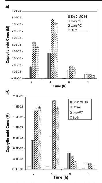
Fig. 7 Caprylic acid concentration obtained upon absorption in the ileum (a) and the jejunum (b) after digestion of tricaprylin in a surfactant-free system (*control*), in the presence of Sn-2 monopalmitin (*Sn-2 MC16*), lysophosphatidylcholine (*LysoPC*) or  $\beta$ -lactoglobulin (*BLG*)
