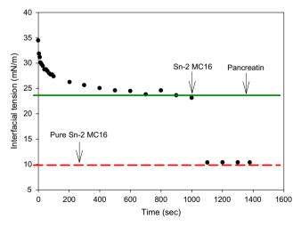
**Fig. 2** Interfacial tension of a buffer/decane system with 10 mg/ml of a crude solution with pancreatic lipase and further injection into the oil phase of  $6.7 \times 10^{-4}$  M of Sn-2 monopalmitin (Sn-2 MC16) after 1,000 s of lipase adsorption
