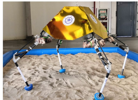
Fig. 2 Structure of a four-legged landing and walking robot.
