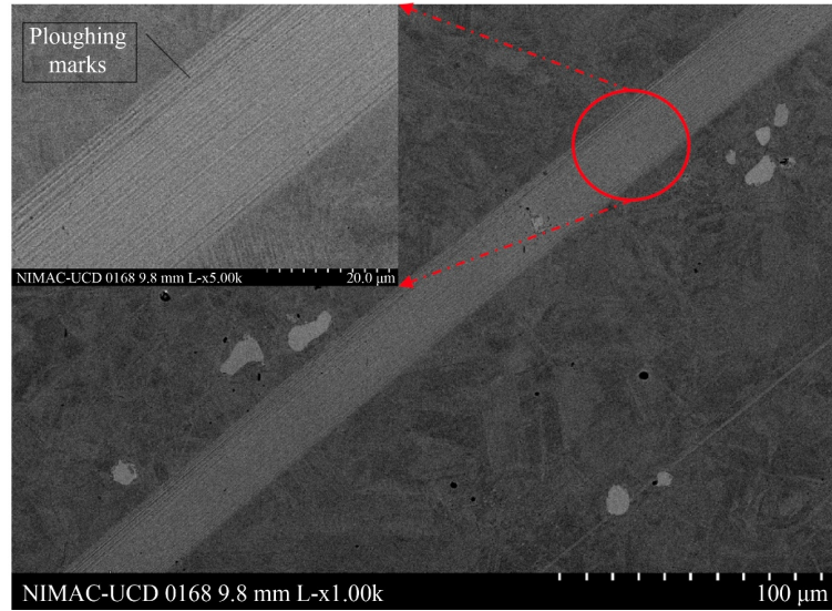
Fig. 9 SEM image of CoCr surface after 10-minute wear under serum-lubricated situation.
