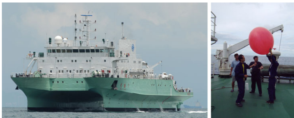
Figure 1 (Color online) ‘ShiYan 1’ Research Vessel (left) and a balloon-borne GPS radiosonde release process (right).
