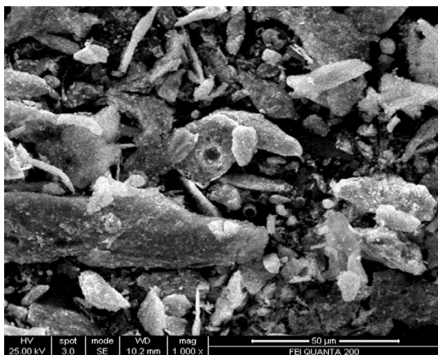
Fig. 4 Scanning electron microscopy (SEM) micrograph showing the morphological characteristics of silver nanoparticles synthesized using the Codium tomentosum leaf extract
