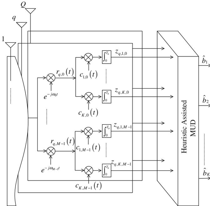
**Fig. 2** MC-CDMA receiver structure considering  $Q$  receive antennas
