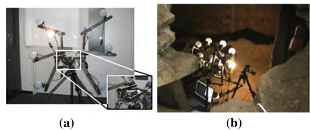
Fig. 4 Photometric-wing system. a RGB camera with six light sources. b Measurement scene using the photometric-wing system
