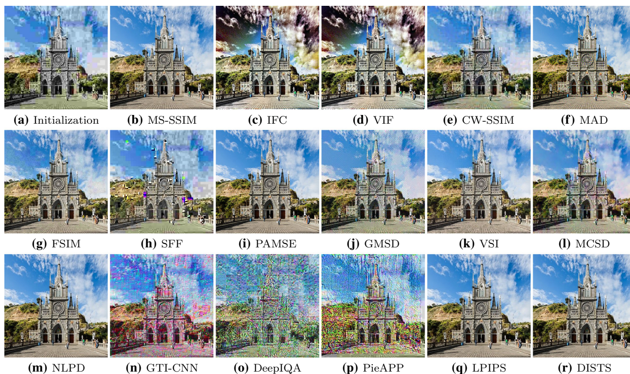
Fig. 2 Reference image recovery test. Starting from (a) a JPEG compressed version of a reference image, we recover images by optimizing the predicted quality relative to the reference image, using different IQA models (b)–(r)
