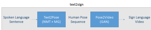
Fig. 4 Full system overview. A spoken language sentence is translated into a representative skeletal pose sequence. This sequence is fed into the generative network frame by frame, in order to generate the input sentence’s sign language translation
