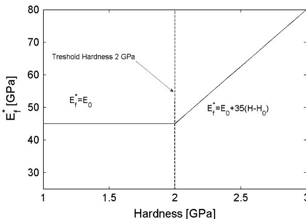
**Fig. 3** Young's modulus of the chemical film as a function of the hardness ( $E = E_0 + 35(H - H_0)$  for  $H > H_0$ ) (e.g. the maximum pressure applied to it). Figure is reproduced using the data presented in [42]
