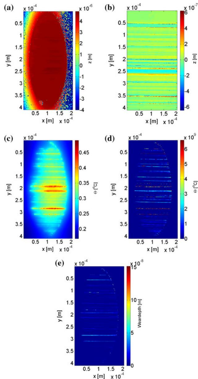
**Fig. 8** **a** Surface profile of a roller run for 8 h under the conditions given in Table 2. **b** Counter surface topography. **c** Temperature field in the contact and **d** Pressure field in the contact. **e** Resulting wear depth
