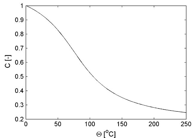
**Fig. 5** Proposed compensation factor  $C[-]$  as a function of the temperature for the yield stress of the chemical reaction layer
