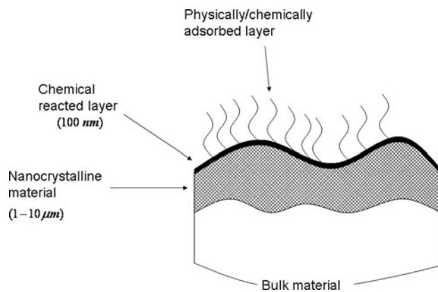
**Fig. 1** Layers present at the surface of a run in system. The *top layer* is a physically/chemically adsorbed layer that only withstands very mild operational conditions. The second layer is a chemical layer that is a mixture of oxides and chemical products of the lubricant. The third layer is a nanocrystalline layer formed at the top of the bulk material by severe plastic deformation under large hydrostatic pressure
