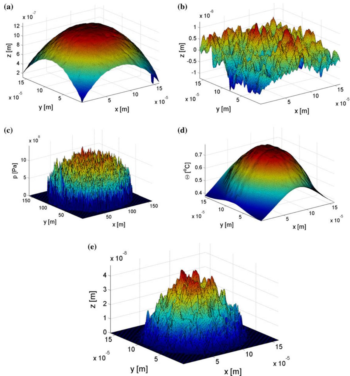
**Fig. 7** **a** Surface topography of the ball and **b** of the disk used during the experiments and simulations. **c** Resulting pressure field and **d** temperature field. **e** Wear volume after 10 m of sliding
