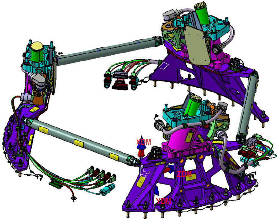
Fig. 3 Main Separation Assembly (MSA), including the interface fittings that remained on the EDM after separation. The EDM is above and TGO is below in the view shown. The separation plane is between the cyan and magenta parts shown above. Each of the three separation mechanisms used a spring release, initiated via a Non-Explosive Actuator (NEA), and incorporated a 128-pin umbilical separation connector. For further details, see Caldirola et al. (2015). Credit: TAS-I/RUAG
