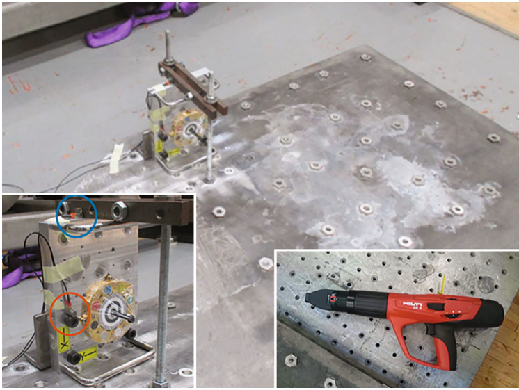
Fig. 27 EQM unit (serial no. 015) mounted on the shock test setup in the “X-axis” configuration. Insert bottom left shows a zoom-in on the target. The blue circle marks the location of the X-accelerator. The orange-red circle marks the Z-accelerator. Insert bottom right shows the Hilti nail gun used to generate the shock
