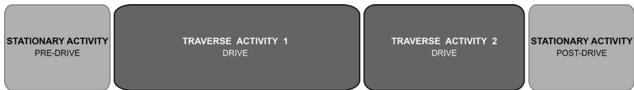
Fig. 19 General graphic representation of a notional RIMFAX drive plan, which includes a single or multiple traverse activities (2 shown here) sandwiched between Pre- and Post-Drive stationary activities
