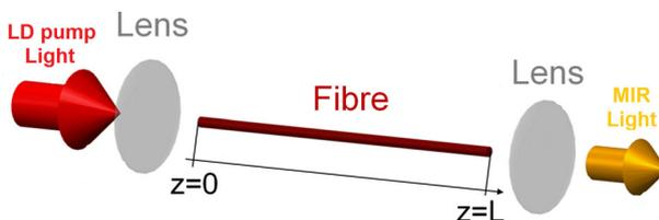
**Fig. 2** Schematic diagram of Tb<sup>3+</sup> doped fibre pumped by a laser diode
