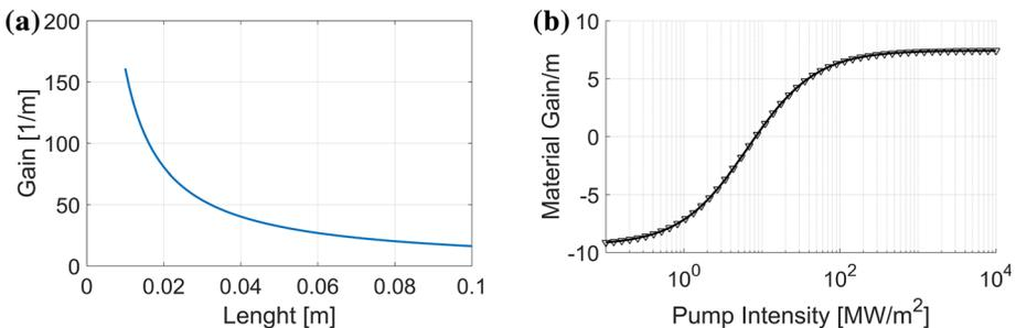
**Fig. 3** Threshold gain dependence on fibre length (a) and gain dependence on pump intensity for  $\text{Tb}^{3+}$ -doped fibre (b)
