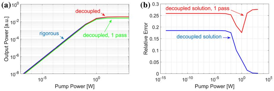
**Fig. 4** The dependence of the output power (a) and the error of decoupled solution (b) on the pump power for a Tb<sup>3+</sup> doped chalcogenide-selenide fibre. The fibre length is 10 cm whilst the fibre end reflectivity is 0.2. The pump wavelength is 2950 nm
