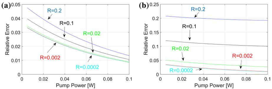
**Fig. 5** The dependence of error of decoupled solution on the pump power calculated at selected values of the fibre end reflectivity R for a Tb<sup>3+</sup> doped chalcogenide-selenide fibre for the approximate algorithm calculating a solution fulfilling the boundary conditions (a) the single pass version of the approximate algorithm (b). The fibre length is 20 mm and the pump wavelength is 2950 nm
