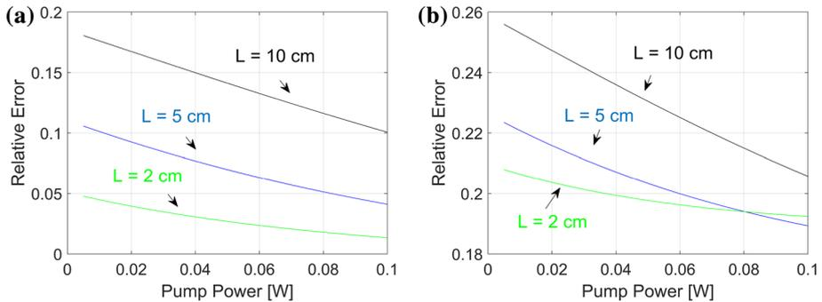
**Fig. 6** The dependence of error of decoupled solution on the pump power calculated at selected values of the fibre length  $L$  for a  $\text{Tb}^{3+}$  doped chalcogenide-selenide fibre, for the approximate algorithm calculating a solution fulfilling the boundary conditions (a) the single pass version of the approximate algorithm (b). The fibre reflectivity is 0.2 and the pump wavelength is 2950 nm
