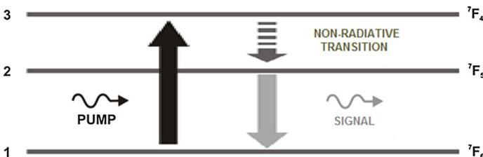
**Fig. 1** Simplified energy level diagram for Tb<sup>3+</sup>
