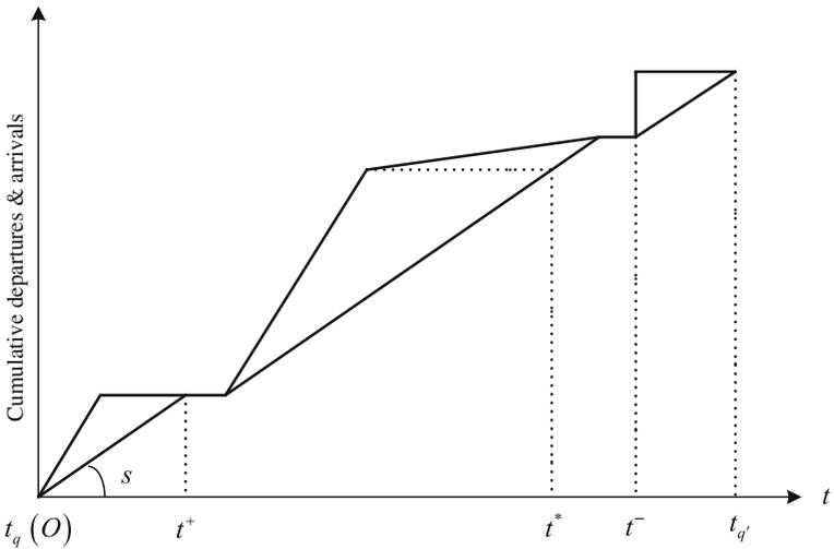
Fig. 5 Profile 4 with capacity waste at both  $t^+$  and  $t^-$
