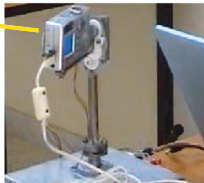
Figure 9. The camera (server side), carried by the robot with two joints, orientates itself according to the orientation of the head “client side”.
