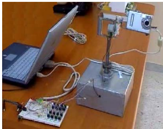
Figure 3. Real diagram of the robot with two joints with its circuit of command.
